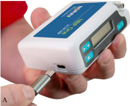
Figure 3: Connecting the NBP One to a PC
